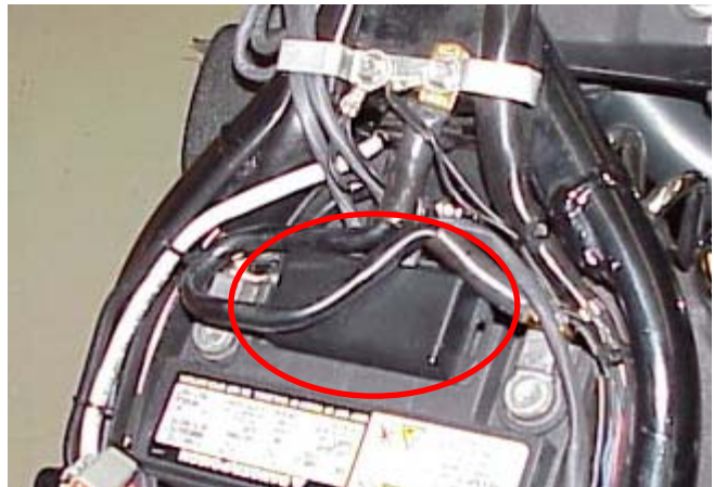
Typical Softail® installation. Mount in the forward pocket on the top of the battery, secure with 2-sided foam tape.
