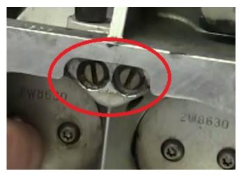
**NOTE:** After Part 2 setup is complete, remove mini usb cable and tighten nuts on ECM caddy. Finish reassembling bike.
