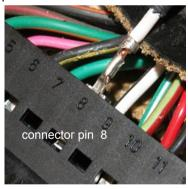
**00-01 models:** Remove screw and slide connector cover off. (pics above). Insert the supplied speed signal wire (single Green / White wire) with the square style terminal into the ECM harness pin slot number 8. Then Install the round terminal end of the speed signal wire in the main harness connector pin location 5 (as shown below)
