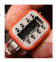
ALL models with mechanical speedo: Install ecm side of green and white wire into ecm terminal 8 (See pic in 95-99). Run wire along existing bike wiring under tank and through fairing. Remove outer fairing, locate the 12 Deutsch connector, it has a white and green wire in terminal 11 on one end and nothing on the other. Unplug connector and release secondary lock. Install the Deutsch pin from the green and white wire into the empty slot in of the connector at terminal 11.
