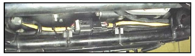
Securely tie harnesses to the frame and/or other harnesses with supplied wire ties. Avoid sharp turns while routing harnesses and avoid areas where engine movement, sharp edges, exhaust systems or hot engine components can contact and cut into the harnesses or connectors.
