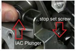
**ALL models:** Check to see if the bellcrank throttle stop is against the stop set screw. If not tighten screw (you may have to heat up to turn) until it just contacts the bell crank throttle stop. Be sure not to over tighten it will move partially open the throttle. If screw turns freely remove, install loctite and readjust until the screw lightly contacts.
