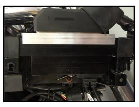
**FL-F:** Route oxygen sensor lead from front pipe along right frame rail and connect to 'front' O2 harness plug. Route front harness connector behind oil filler spout. Position connector along lower frame rail between engine and transmission. Push the 2 connectors together and listen for a loud "CLICK".
