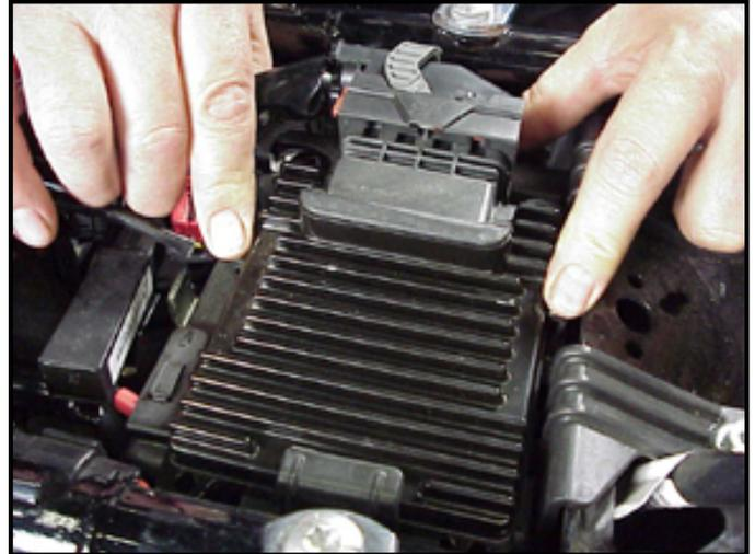
**Step 3** Disconnect the ECM from the connector as per the following procedure:
