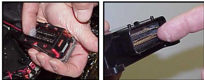
Before connecting, verify that the locking bar is in the fully open, rearward position (locking bar index pin is fully engaged with rear notch in the socket housing).
