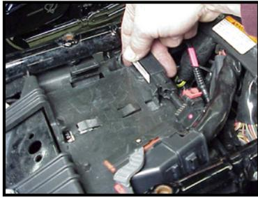
**Step 5** Install main harness connector to ThunderMax ECM. Before installing connector, lightly spread some dielectric grease (included in package) on harness connector terminals, and on the inside lip of the connector port opening of the ECM to allow the rubber weather seal in the connector plug to slide into place without binding. See 'Tips' on page 7 for additional dielectric grease instructions.
