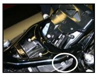
**Step 2k** Secure harnesses away from hot or moving parts using supplies wire ties. Re-install main fuse, seat and seat pan/fender assembly.
