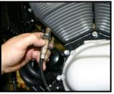
**Step 2i** Route rear O<sub>2</sub> sensor and AutoTune power harness between left frame rail and oil tank. Install O<sub>2</sub> sensor into rear exhaust pipe and connect plug. Plug AutoTune power harness into 4-pin (gray) data port plug as shown.
