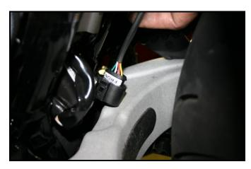
**Step 2h** Route front  $O_2$  sensor from under transmission through gap between lower frame rail and primary cover, along frame rail to front exhaust pipe. Carefully wind  $O_2$  sensor harness 3-4 turns counterclockwise before installing into exhaust pipe; turn clockwise while installing to unwind harness. Connect harness plug.
