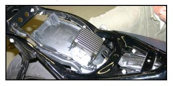
**Step 2d** Install the ThunderMax ECM to the inner fender using (2) 6mm x 20mm socket head screws supplied. Route wires as shown.
