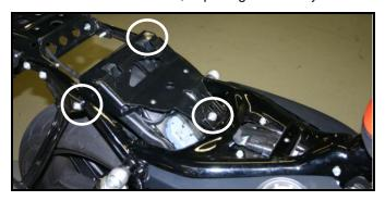
**Step 2c** Remove the lower inner fender bolt and allow the inner fender to rest on the rear tire. Unplug and remove the factory ECM from the inner fender.
