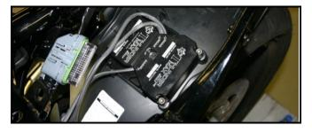
**Step 2e** Install ThunderMax Pigtail connector # 309-324 to 36 pin harness connector per connector instructions.
