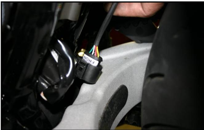
**Step 2h** Route front O<sub>2</sub> sensor from under transmission through gap between lower frame rail and primary cover, along frame rail to front exhaust pipe. Carefully wind O<sub>2</sub> sensor harness 3-4 turns counterclockwise before installing into exhaust pipe; turn clockwise while installing to unwind harness. Connect harness plug.
