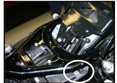
**Step 2k** Secure harnesses away from hot or moving parts using supplies wire ties. **Re-install main fuse,** seat and seat pan/fender assembly.
