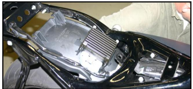
**Step 2d** Install the ThunderMax ECM to the inner fender using (2) 6mm x 20mm socket head screws supplied. Route wires as shown.
