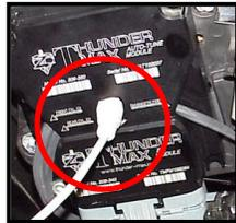
**Special Note for International Model Bikes with Active Exhaust Enabled:** *If your bike is equipped with a working Active Exhaust Valve, you must unplug the active exhaust harness before linking to the module, as the AEV circuitry conflicts with the communication stream. You can re-connect the harness after unlinking. If the stock exhaust has been changed, disregard this step. ThunderMax does not support active exhaust*
