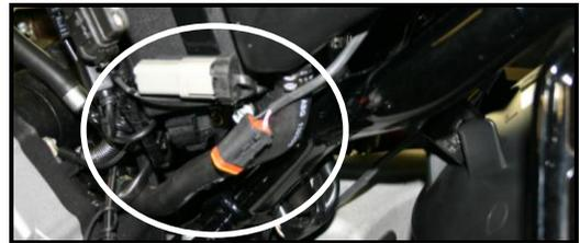
**Step 2j** Route Pigtail harness connector to top of frame triangle in front of left side shock for easy access under left frame cover. Re-mount inner fender and steel frame bracket with ECM attached.
