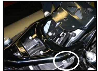
**Step 2k** Secure harnesses away from hot or moving parts using supplies wire ties. **Re-install main fuse,** seat and seat pan/fender assembly.
