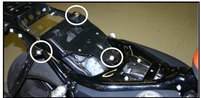
**Step 2c** Remove the lower inner fender bolt and allow the inner fender to rest on the rear tire. Unplug and remove the factory ECM from the inner fender.
