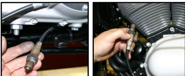
**Step 2i** Route rear O<sub>2</sub> sensor and AutoTune power harness between left frame rail and oil tank. Install O<sub>2</sub> sensor into rear exhaust pipe and connect plug. **Plug AutoTune power harness into 4-pin (gray) data port plug as shown.**
