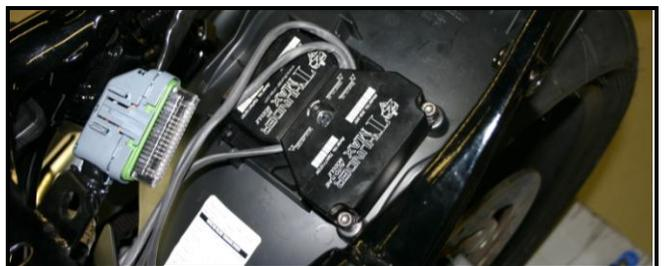
**Step 2e** Install ThunderMax Pigtail connector # 309-324 to 36 pin harness connector per connector instructions.
