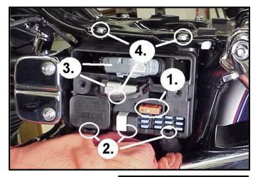
**FXD-B:** Remove the stock ECM from the electrical caddy. The caddy must be slightly modified for additional main harness connector clearance.
