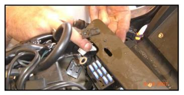
**ST-C:** Connect the ThunderMax 50 ECM to the harness and position it loosely in the ECM tray. Feed both oxygen sensor harnesses (front cylinder first) through the gap between the frame and oil tank on the right side of the motorcycle.
