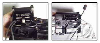
**FXD-D:** Feed the front cylinder oxygen sensor harness through to the right side of the bike, over the top and to the rear of the starter motor. Reinstall the caddy with fuse and relay blocks in place. Reconnect the TSSM, coil and ECM harnesses and main fuse. Plug the AutoTune module plug into the data link on the bike. It is through the data port that data from the AutoTune
