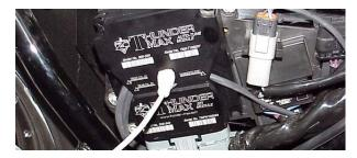
**Step 7** To link to the module, turn the key switch to the "Ignition" position, making certain the "RUN / OFF" rocker switch (Kill Switch) on the handlebar controls is in the "RUN" position. Select the "Link" Button in the SmartLink software. The button turns green to indicate a successful link. Answer **[No]** to the "Do you wish to READ the module map now" question at this time.
