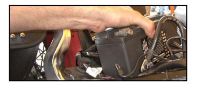
**ST-B:** Remove the bolts holding the fuse block bracket to the frame and lift the bracket away from the frame to allow access to the gap between the frame and oil tank on the right side of the motorcycle.
