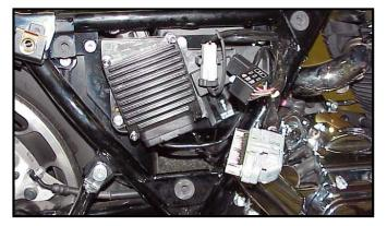
**FL-C:** Install the ECM wiring harness to the ThunderMax 50 ECM. Do not install the ECM onto the motorcycle at this point. If the ECM is mounted onto the electrical caddy at this step, it is difficult to get the fuse box in place.
