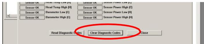
When the Diagnostic Codes window appears, select [Clear Diagnostic Codes]. After completing this step, select Basic Settings from the Module Configuration menu and verify that the speedometer calibration is correct. After verifying these settings, click **[Write Basic Settings]**.
