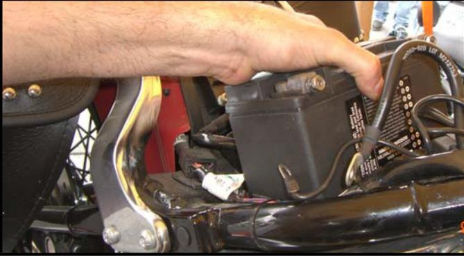
**ST-B:** Remove the bolts holding the fuse block bracket to the frame and lift the bracket away from the frame to allow access to the gap between the frame and oil tank on the right side of the motorcycle.
