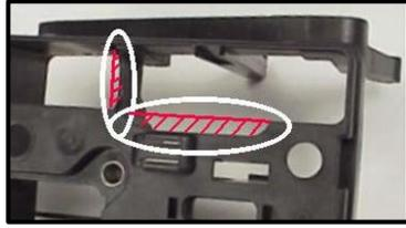
Use a Dremel or Roto-Zip tool to provide additional clearance for the harness plug catch; also remove approximately 3/8" from the partition support as shown.
