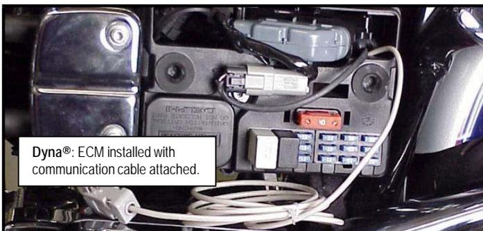
Dyna®: ECM installed with communication cable attached.
