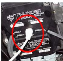
**Step 6** To link to the module, turn the key switch to the "Ignition" position, making certain the "RUN / OFF" rocker switch (Kill Switch) on the handlebar controls is in the "RUN" position. Select the "Link" Button in the SmartLink software. The button turns green to indicate a successful link. Answer **[No]** to the "Do you wish to READ the module map now" question at this time.
