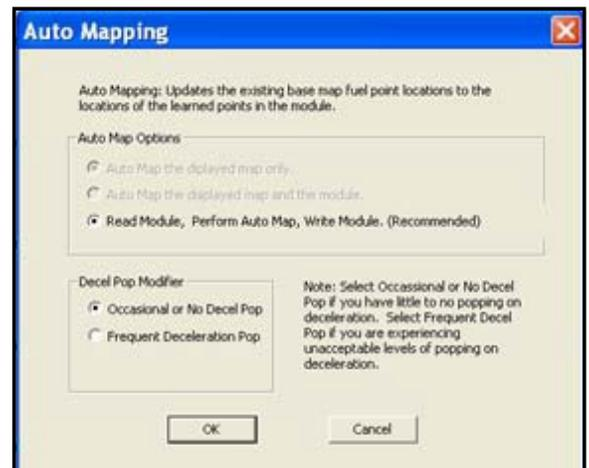
The adjusted fuel points will be automatically smoothed and the base map re-written with the new, optimized fuel points. Save the modified map to your hard drive before unlinking, and go ride!
