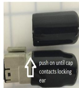
**H-D® released a Tech Tip (#418)** regarding improving conductivity at the throttle body wire connector (TCA). Carefully remove the harness plug from the throttle body, clean the male TCA pins with a swab and alcohol, apply dielectric grease to the female terminals and reassemble.
