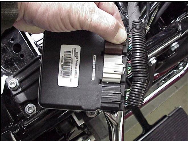
**FL-G:** With the factory ECM removed, route the AutoTune harness thru the opening on right side of the frame below the down tube for the seat, towards the ECM caddy.
