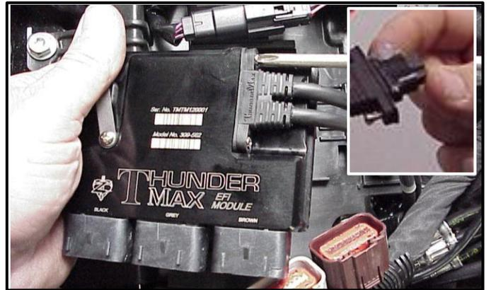
**FL-I:** Install main harness connectors to ThunderMax ECM. Before installing the connectors, lightly spread some dielectric grease on harness connector terminals.
