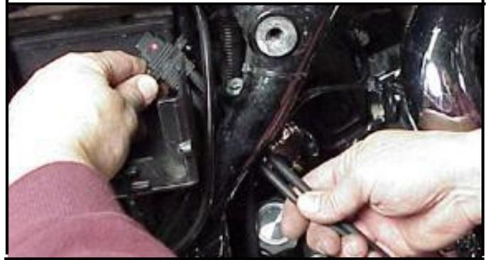
**FL-H:** Route the AutoTune harness plug under the brake lines to the ECM caddy area. Locate the package of dielectric grease included with communication cable. Spread a small amount of grease on the AutoTune harness plug end and inboard of the mounting flange to allow the plug to easily slide into the ThunderMax ECM. Install in case with the ThunderMax logo up and attach with the provided screws.
