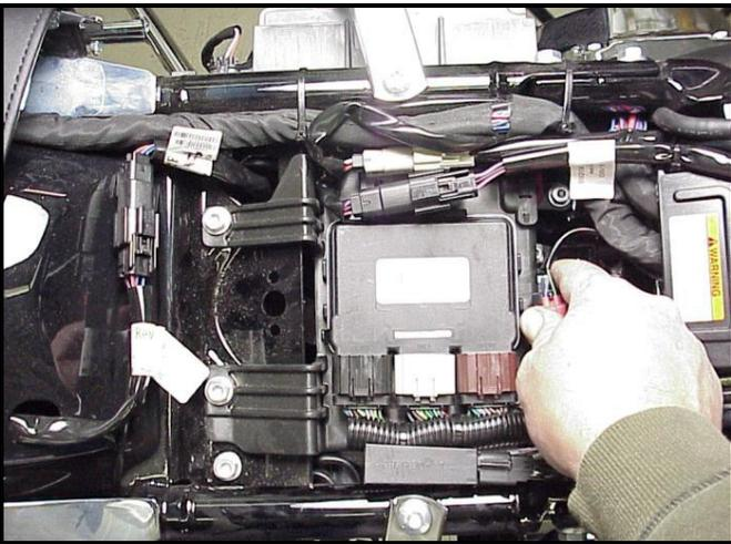
**FL-F:** Disconnect the ECM from the three connectors by depressing the tab on the top of each connector. Some models have a red locking slide on the connectors. If equipped the red lock must be slid outward towards the harness before the the connector tab is depressed.
