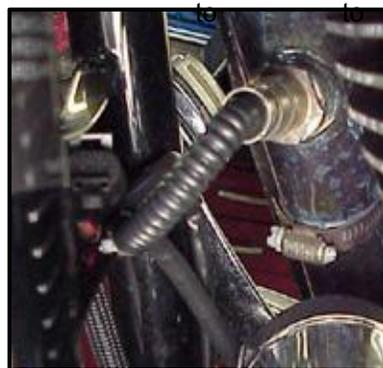
Bungs should be located no more than 3 - 4” from the head pipe connection (for ideal location, refer to the factory location on 2009 models). Weld-in bungs are available from many sources in straight or angled designs.
