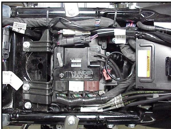
**FL-K:** Connect the oxygen sensor harnesses to the AutoTune harness, you will hear a click when they are connected properly. Carefully wire tie the leads to the motorcycle. Take extra care to ensure harness and sensor leads are safe from rubbing or chaffing on the motorcycle. Use all supplied wire ties; add extra ties if needed to properly secure wiring on your installation.
