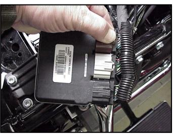
**Step 4** If equipped with factory alarm, detach alarm antenna from ECM caddy clip by lifting slightly and sliding to the right of the bike – do not disconnect wiring.
