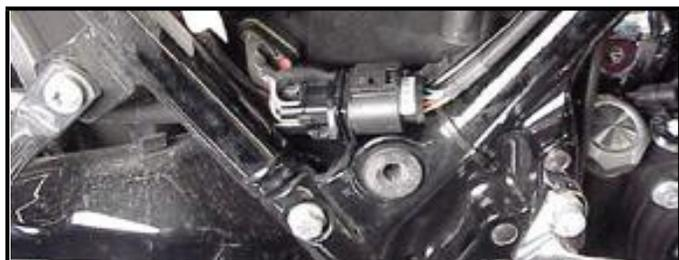
**FL-M:** Position front connector above lower frame rail between engine and transmission. Attach to existing harness with provided wire ties. Inspect all wiring to make sure it is clear of moving parts and excessive heat.
