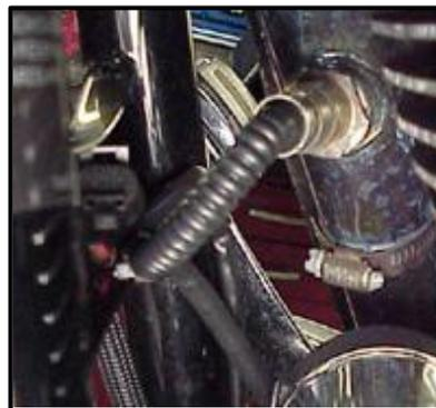
Bungs should be located no more than 3 - 4” from the head pipe connection (for ideal location, refer to the factory location on 2009 FL models). Weld-in bungs are available from many sources in straight or angled designs.
