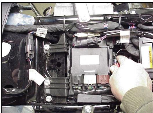
**FL-F: 309-588** Disconnect the ECM from the three connectors by depressing the tab on the top of each connector. Some models have a red locking slide on the connectors. If equipped the red lock must be slid outward towards the harness before the the connector tab is depressed.
