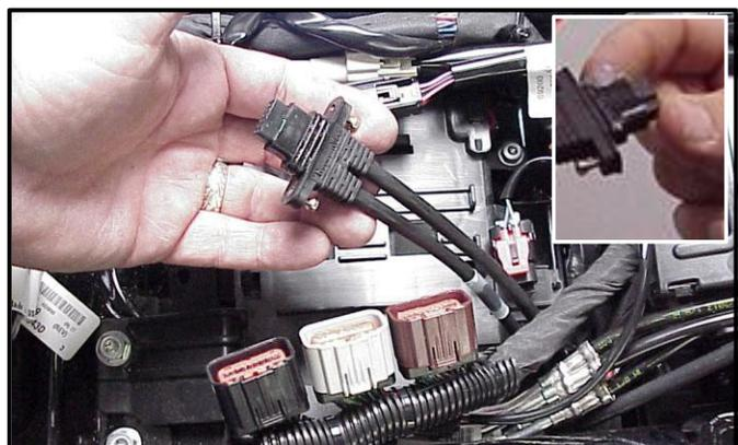
**FL-I:** Install main harness connectors to ThunderMax ECM. Before installing the connectors, lightly spread some dielectric grease on harness connector terminals.
