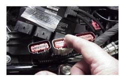
**Step 6** Place the ThunderMax ECM into the ECM caddy. If equipped, position alarm antenna as shown.
