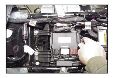
**Step 3** Disconnect the ECM from the three connectors by depressing the tab on the top of each connector.
