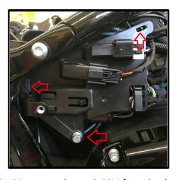
**Step 3** Disconnect the stock ECM from the three connectors by depressing the tab on the top of each connector. Slide ECM towards the front of the bike to remove from the electrical caddy.
