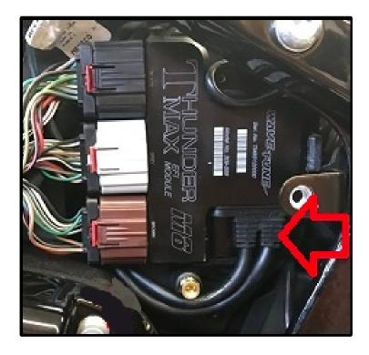
shown with 309-UXM Wide Band upgrade harness installed. 309-589-X will have a silver block off plate at this location.
