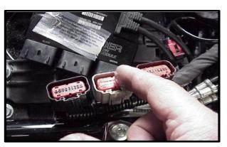
**Step 4** Install main harness connector to ThunderMax ECM. Before installing connector, lightly apply some dielectric grease (included in package) on harness connector terminals, and on the inside lip of the connector port opening of the ECM to allow the rubber weather seal in the connector plugs to slide into place without binding. 'Tip' Also apply Dielectric grease to the TAC connector on the side of the Throttle Body.
