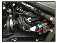
Special Note – If you have previously installed another tuning device such as a Power Commander, be sure to remove the device and any "O2 Sensor Eliminators" that may have been installed at the sensor harness plugs at that time!
