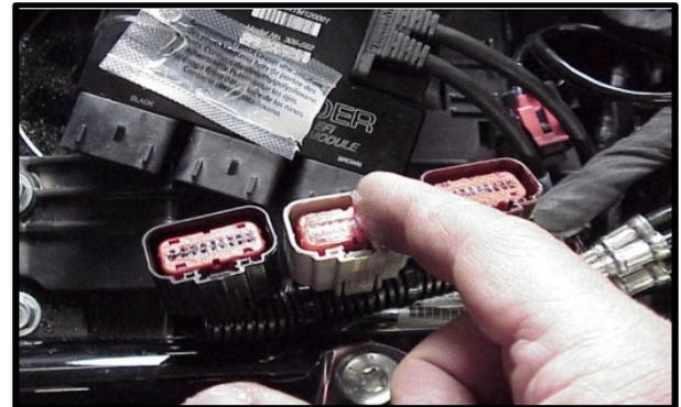
**Step 4** Install main harness connector to ThunderMax ECM. Before installing connector, lightly apply some dielectric grease (included in package) on harness connector terminals, and on the inside lip of the connector port opening of the ECM to allow the rubber weather seal in the connector plugs to slide into place without binding. 'Tip' Also apply Dielectric grease to the TAC connector on the side of the Throttle Body.
