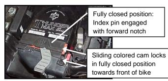
**Important Note:** Pin and socket housing of the connector must be fully engaged before you rotate the locking bar to the forward position. Forcing the locking bar forward before the connector is fully engaged will damage the connector and/or the ECM
