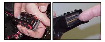
Before connecting, verify that the locking bar is in the fully open, rearward position (locking bar index pin is fully engaged with rear notch in the socket housing).
