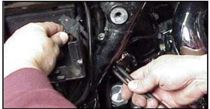
**H:** If equipped with factory alarm, detach alarm antenna from ECM caddy clip by lifting slightly and sliding to the right of bike (do not disconnect).
