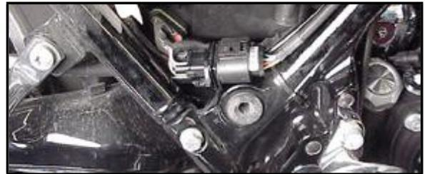
**N:** Position front connector above lower frame rail between engine and transmission. Attach to existing harness with provided wire ties. Inspect all wiring to make sure it is clear of moving parts and excessive heat.
