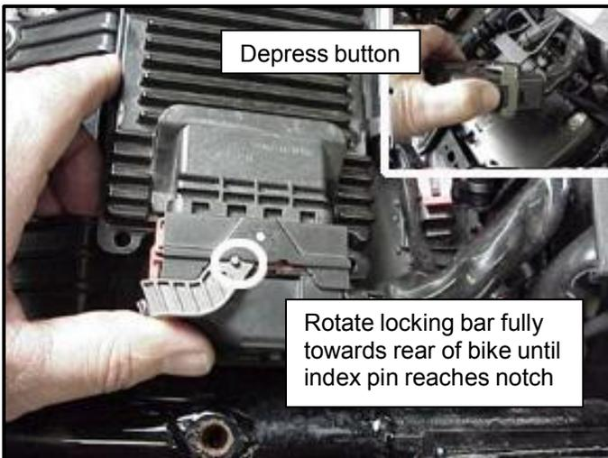
The connector internal latches are not fully disengaged until the locking bar on the connector is seated to the full rearward position to complete removal of the connector. If you force the socket housing with latches partially engaged, it will result in damaging the connector. Once index pin is fully seated, with steady yet careful attention, pull apart the connector from the factory ECM and remove it from the motorcycle.
