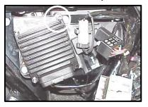
FL-C: Remove the factory ECM from the motorcycle, the ECM is held to the electrical caddy by head socket cap The screws screws. have a locking agent on them and can be difficult to remove.
