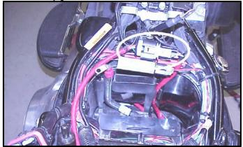
**FX/FLST-K:** Route front oxygen sensor harness behind and under transmission with connector plug just under the engine/transmission mounting boss; connect to front oxygen sensor.
