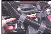
XL-B Remove the left side cover, locate and remove ECM the Power fuse. Remove the seat. unplug and remove the factory ECM. Feed the ThunderMax oxygen
