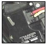
FL-E: Insert the greased oxygen harness connector into the ECM with the imprinted "ThunderMax" logo facing up. (2) Tighten the Phillips connector screws. Install the ThunderMax ECM to the ECM caddy using original screws.
