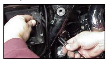
**FL-H:** Route the AutoTune harness plug under the brake lines to the ECM caddy area. Locate the package of dielectric grease included with communication cable. Spread a small amount of grease on the AutoTune harness plug end and inboard of the mounting flange to allow the plug to easily slide into the ThunderMax ECM. Install in case with the ThunderMax logo up and attach with the provided screws.
