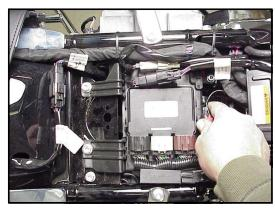
**FL-F: 309-588** Disconnect the ECM from the three connectors by depressing the tab on the top of each connector. Some models have a red locking slide on the connectors. If equipped the red lock must be slid outward towards the harness before the the connector tab is depressed.
