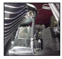
**FL-E:** Remove factory ECM located under the seat from the caddy by spreading the plastic caddy latches at the sides of the ECM. Lift the ECM up and to the right to release it from the caddy.
