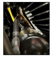
Bungs should be located no more than 3 - 4" from the head pipe connection (for ideal location, refer to the factory location on 2009 FL models). Weld- in bungs are available from many sources in straight or angled designs. See Video on adding new bungs on the web at Youtube.com (search ThunderMax bung).
