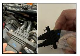
**FL-I:** Install main harness connectors to ThunderMax ECM. Before installing the connectors, lightly spread some dielectric grease on the harness connector terminals.
