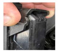
**FL-G:** Route rear O2 sensor plug through the opening at the right side of the frame below the branch of harness going to the left side of the bike into the area just below the ABS module. Then feed the ECM harness plug through the same opening upward towards the left side in front on the battery.
