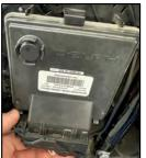
**FL-F:** Disconnect the ECM from the harness connector by depressing the harness cover inward slightly. hile pressing inward, gently raise the latching arm and slide it to the left to fully unlatch the connector.
