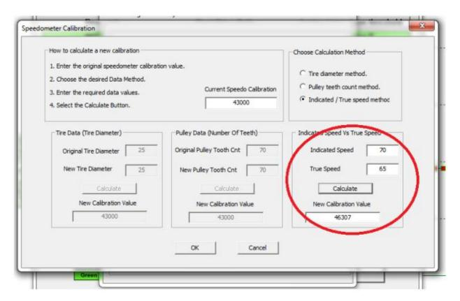
As you OK and exit this series of dialogs, you will see the NEW calibration value has been stored in the basic setting. It has also been stored in the Module.
