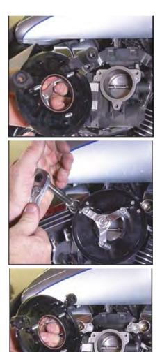
"DISCLAIMER: NOT LEGAL FOR SALE OR USE IN CALIFORNIA ON ANY POLLUTION CONTROLLED MOTOR VEHICLES" **Step 2d** Start the 4 - #10 button head cap screws through the backing plate into the breather housings. Snug the 4 - #10 bolts prior to being tight, insert the breather housing cap into the breather housing, then tighten the (4) #10 bolts. Now tighten the (3) 1/4" filter mount to throttle body bolts.
