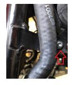
b. Gently pull outward on cooler, slide fan assy upward into place (notch is the top side)
