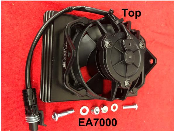
b. Gently pull outward on cooler, slide fan assy upward into place (notch is the top side)
