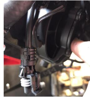
c. Remove connector plug from bike fan harness, plug the fan connector in.
