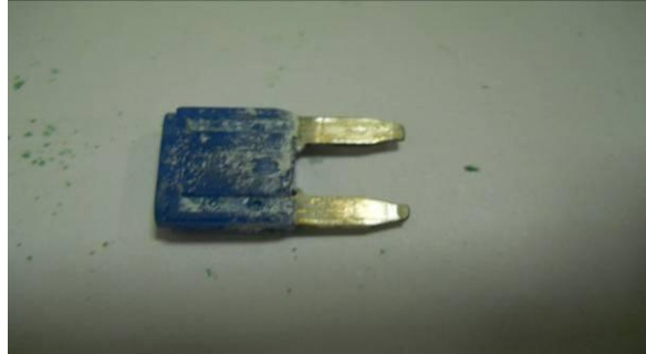
Note- corrosion / scale on spades
