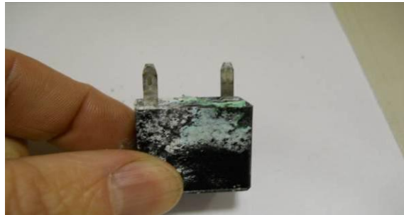
Replace severely corroded parts
