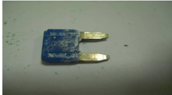
Note- corrosion / scale on spades
